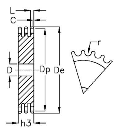
C = 1 D = 20 De = 201.6 Dp = 197.15 For chain size =  $3/8 \times 7/32$ For chain type = 06 B-3 h3 = 25.6
